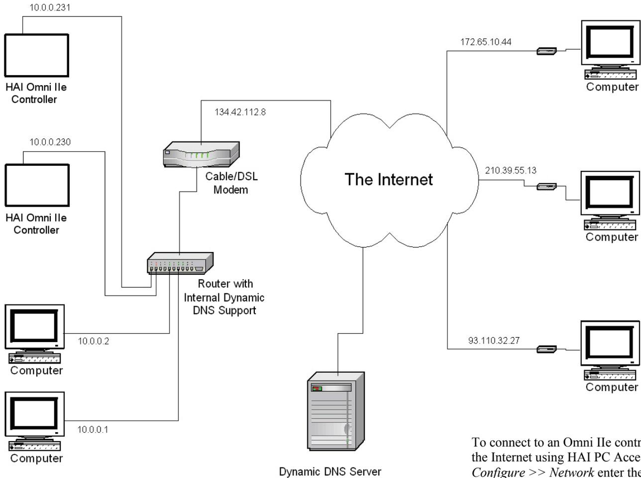
To connect to an Omni IIE controller on a local network using HAI PC Access, under *Configure >> Network* enter the controller's IP address:
